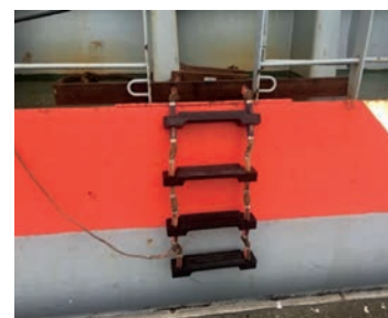
A spreader used for securing the ladder behind a very thin piece of railing.
