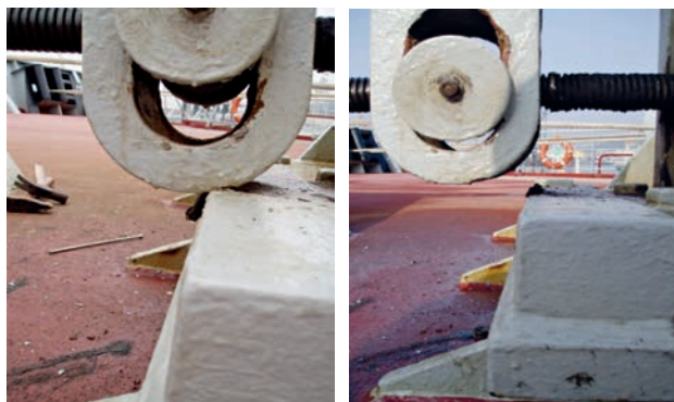
Incorrect Brake Adjustment Correct Brake Adjustment
