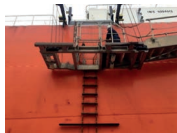
Non-compliant trapdoor arrangement.
