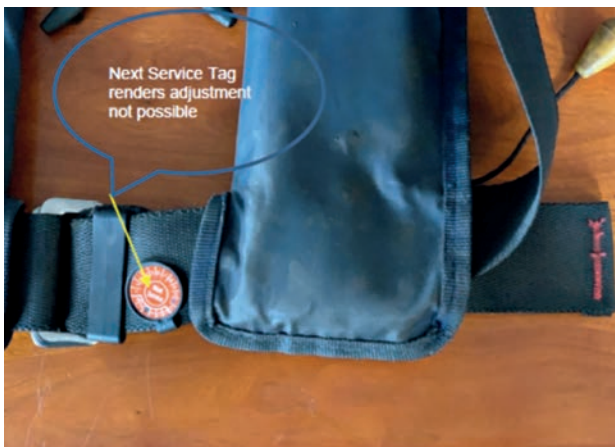
Highlighting that the positioning of the service tag renders waist strap adjustment impossible
