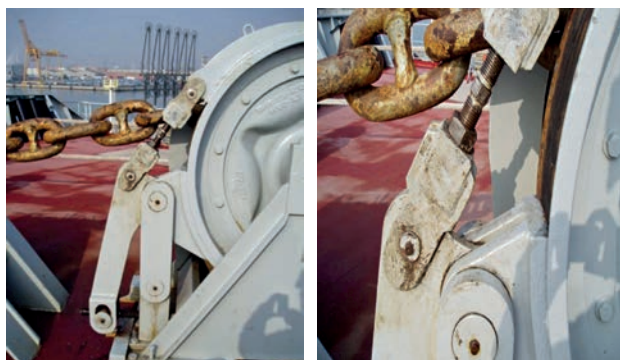
Brake ‘Fully On’ Bottle Screw Adjustment
